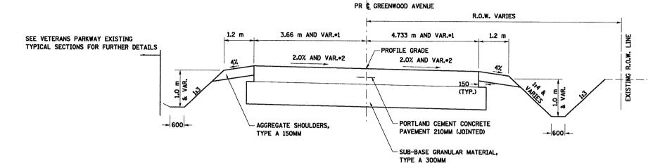
•1 VARIES FROM 3.66 m LT & 4.733 m RT AT STA. 6+989.437 TO 4.5 m AT STA. 7+024.475 •2 2.0% FROM STA. 6+989.437 TO STA. 7+010.000 VARIES FROM 2.0% AT STA. 7+010.000 TO 3% AT STA. 7+024.475
