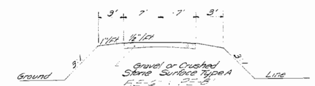
DETAIL OF FIELD AND PRIVATE ENTRANCE SECTION A-A
