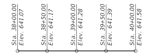
GRINNELL ROAD PROFILE GRADE (Along centerline roadway)
