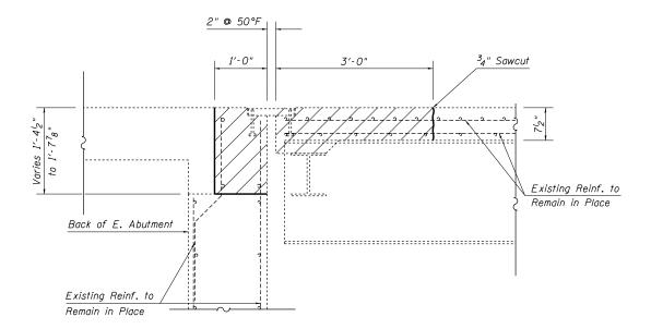
SECTION A-A (Dimensions at Rt. L's to end of deck) (EAST ABUTMENT)
