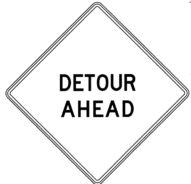
W20-2 MIN; 48.0" across sides 2.3" Radius, 0.9" Border, 0.6" Indent, Black on Orange; [DETOUR] D 60% spacing; [AHEAD] D 102% spacing;
