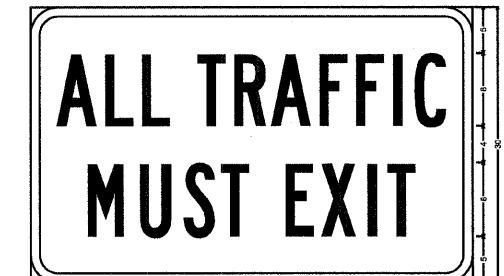
M3-6 MIN & STD; 1.5" Radius, 0.6" Border, 0.4" Indent, Black on White; [ALL] B 2K 85% spacing; [TRAFFIC] B 2K 85% spacing; [MUST] B 2K; [EXIT] B 2K; Table of widths and spaces:
