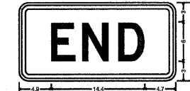
M3-5 MIN & STD; 1.5" Radius, 0.6" Border, 0.4" Indent, Black on Orange; [END] D 2K; Table of widths and spaces:
