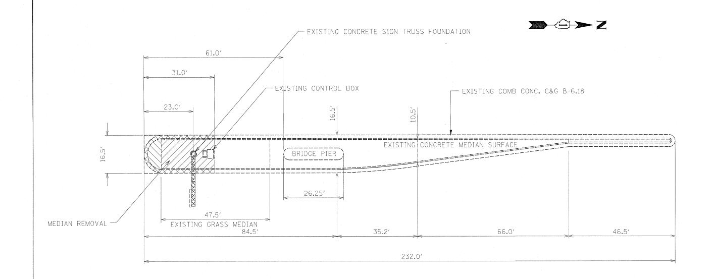
NOTE: THE REMOVAL OF EXISTING COMBINATION CONCRETE CURB AND GUTTER, TYPE B-6.18, CONCRETE MEDIAN NOSE, SOD AND TOPSOIL AS SHOWN ON THE PLANS SHALL BE PAID FOR AT THE UNIT PRICE PER SQUARE FOOT FOR "MEDIAN REMOVAL."
