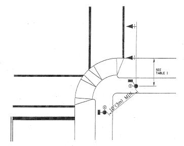
RECOMMENDED PUSHBUTTON LOCATIONS FOR ACCESSIBLE PEDESTRIAN SIGNALS SHALL BE IN ACCORDANCE WITH THE CURRENT MUTCO (SEE NOTE 1). TO MEET MUTCD REQUIREMENTS, PEDESTRIAN SIGNAL PUSHBUTTONS MAY HAVE TO BE MOUNTED ON A SEPARATE POST.
