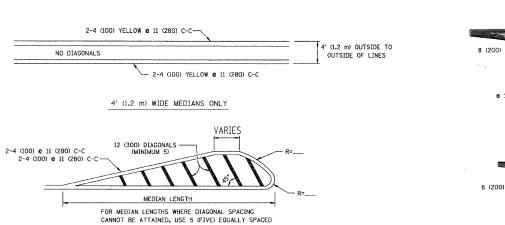
DIAGONAL LINE SPACING: 50' (15 m) C-C (LESS THAN 30MPH (50 km/h))
