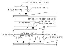
\*\* TURN LANES IN EXCESS OF 400' (120 m) IN LENGTH MAY HAVE AN ADDITIONAL SET OF ARROW - "ONLY" INSTALLED MIDWAY BETWEEN THE OTHER TWO SETS OF ARROW - "ONLY".
