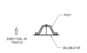
DELINEATORS SHALL BE INSTALLED ACCORDING TO STANDARD 635001 EXCEPT THAT THE POST SHALL BE ROTATED 180°. THE POST WILL HAVE THE WIDE SIDE FACING TRAFFIC AND THE DELINEATOR ATTACHECD AS SHOWN ABOVE.
