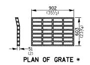
\* THIS GRATE TO BE USED WITHOUT CURB BOX WHEN INLET IS IN DRIVEWAY.
