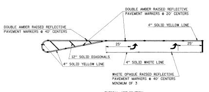
TYPICAL APPLICATION FOR LEFT TURN LANE WITH RAISED REFLECTIVE PAVEMENT MARKERS
