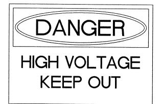
PROVIDE WARNING SIGN ON VAULT EXTERIOR DOORS LABELED "DANGER - HIGH VOLTAGE - KEEP OUT" PER THE REQUIREMENTS OF NEC 110.34 (C).
