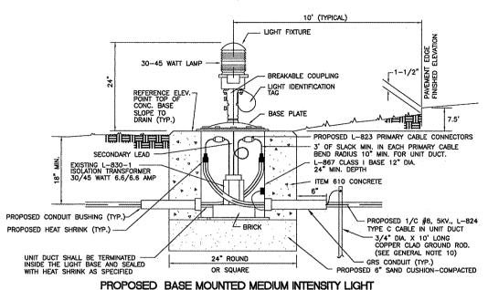
10' (TYPICAL) LIGHT FIXTURE -30-45 WATT 1" THIN WALL COLUMN LIGHT IDENTIFICATION REFERENCE ELEVATION POINT TOP OF STAKE SECONDARY LEADER 1-1/2" SAND OR COMPACTED-EARTH BACKFILL -1/C #8, 5KV., L-824 TYPE C CABLE IN 3/4" UNIT DUCT (TYP.) ISOLATION TRANSFORMER -/ 6.6 AMP 30-45 WATT (L-830-1) HEAT SHRINK (TYP.) 3/4" DIA. X 10' LONG COPPER CLAD GROUND ROD. (SEE ELECTRICAL GENERAL NOTE 10) 30" ANGLE IRON STAKE CONCRETE ANCHOR (COST INCIDENTAL)
