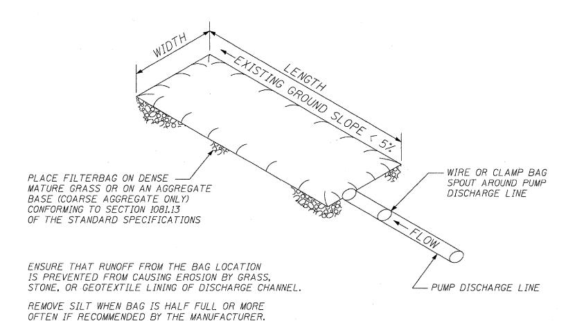
DİSPOSE OF SILT BY TRANSPORTING THE FILLED BAG TO DISPOSAL AREA. SLIT THE BAG, BLEND SILT INTO EXISTING TOPOGRAGHY, SEED AND MULCH
