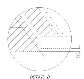
Existing reinforcement extending into the removal area shall be cleaned, straightened and incorporated into the new construction. Any reinforcement that are damaged during concrete removal shall be replaced with an approved splicer or anchorage system. Cost shall be included with Concrete Removal. Hatched areas indicate Concrete Removal.
