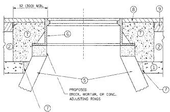
EXISTING BROKEN FRAMES AND LIGS SHALL BE REMOVED AND DISPOSED OF BY THE CONTRACTOR AND SHALL BE REPLACED AS DIRECTED BY THE ENGINEER. REPLACEMENT FRAMES AND LIDS WILL BE PAID FOR IN ACCORDANCE WITH ARTICLE 109.04 OF THE STANDARD SPECIFICATIONS UNLESS A SEPARATE PAY ITEM HAS BEEN PROVIDED.
