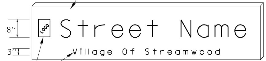
LED ILLUMINATED SIGN PANEL 8'0 x 2'6" (750 mm x 2.5 mm)(MAX) C or D FONT
