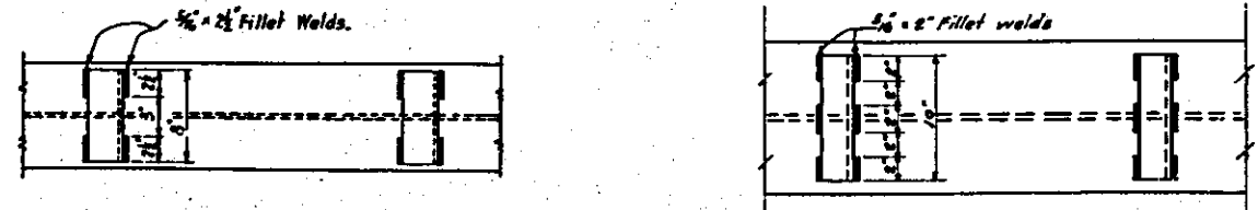
TOP VIEW SHOWING WELDING OF LUGS TO BEAM IN SPAN 1
