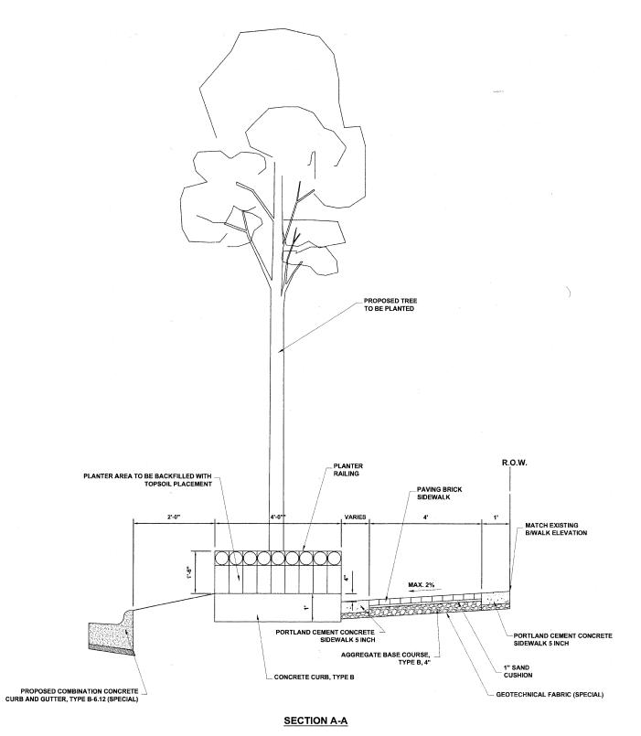
PORTLAND CEMENT CONCRETE SIDEWALK 5 INCH PAVING BRICK SIDEWALK PORTLAND CEMENT CONCRETE SIDEWALK 5 INCH - CONCRETE CURB, TYPE B PROPOSED TREE TO BE PLANTED PLANTER RAILING WITH BASE PLATE
