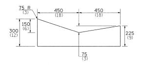
THIS WORK SHALL BE DONE IN ACCORDANCE WITH THIS DETAIL AND STANDARD 606101 THIS WORK SHALL BE PAID FOR AT THE CONTRACT UNIT PRICE PER METER (FOOT) FOR CONCRETE GUTTER, TYPE A (SPECIAL).
