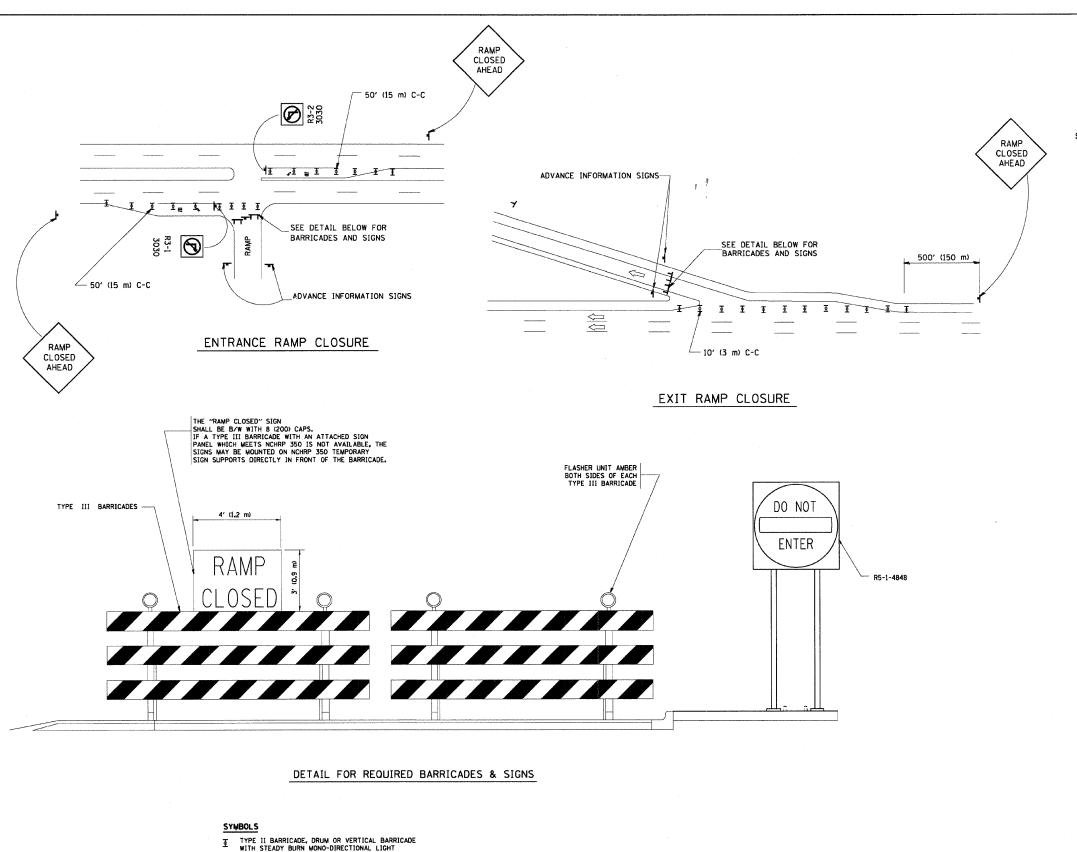
TYPE III BARRICADE WITH FLASHING LIGHT
