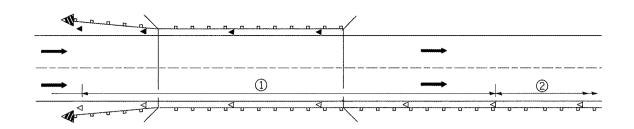
① Spacing 80 ft. (24 m) max. for first 400 ft. (122 m) or curve spacing shown in Standard 635001, whichever is less (min. 4 reflectors regardless of length).
