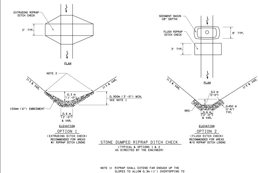
SLOPES TO ALLOW 0.3m (1') OVERTOPPING TO AVOID ERODING AROUND THE EDGES OF THE
