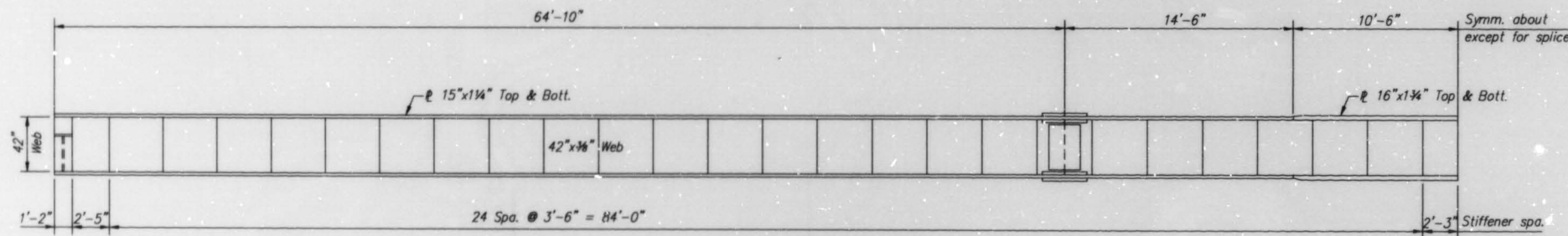
HALF GIRDER ELEVATION (EXISTING)
