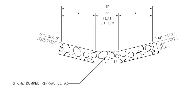
DETAIL OF STONE DUMPED RIPRAP, CLASS A3
