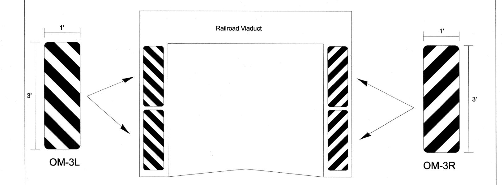
Sign panels to be placed as shown on both sides of the railroad viaduct and to be attached to the structure to the satisfaction of the Engineer.
