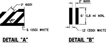
TYPICAL CROSSWALK MARKING
