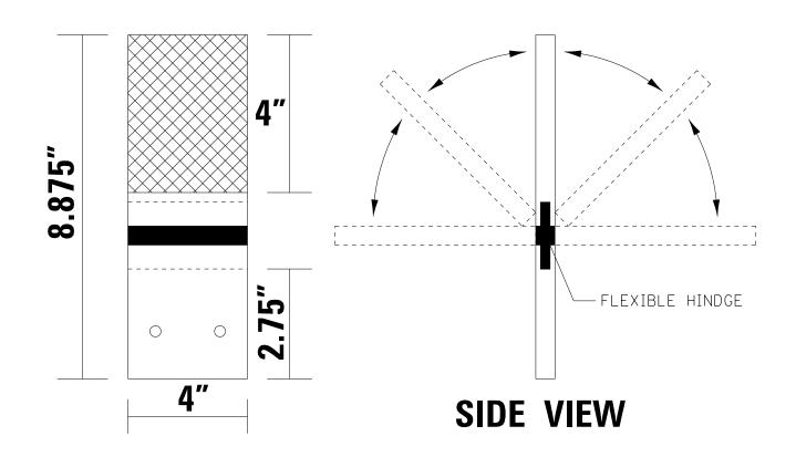
REFLECTORS MAY BE MOUNTED DIRECTLY TO METAL, WOOD OR PLASTIC BLOCK OUTS.
