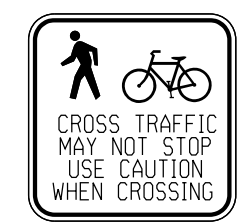
CROSS TRAFFIC MAY NOT STOP USE CAUTION WHEN CROSSING SIGN (12" x 12") PEDESTRIAN SYMBOL HEIGHT - 4" (IN) BICYCLE SYMBOL HEIGHT - 3" (IN) LETTERS - 1" C LEGEND - BLACK BACKGROUND - YELLOW
