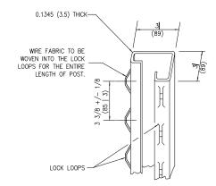
**ROLL FORMED SECTION OF** TERMINAL + GATE POST
