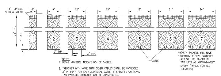
3. DEPTH OF TRENCHES SHALL BE AS SHOWN ABOVE UNLESS OTHERWISE SPECIFIED ON THE PLANS.
