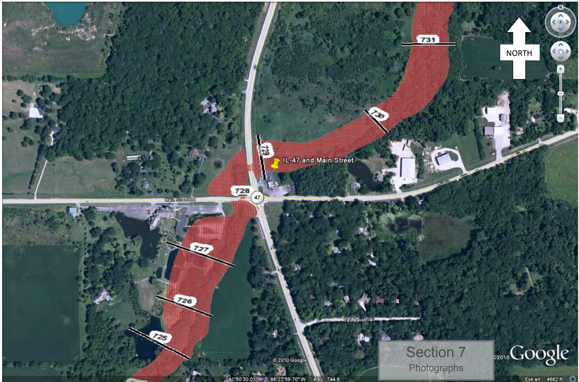
Google Earth View with FEMA Floodway (Hatching) and FEMA known BFE's shown. Aerial Photo Date 2009
