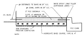
SET 3/4" WHITE EPOXY EXPANSION JOINTS AT POINTS ABUTTING CURB OR PAYEMENT AND AT 60" MAX. INTERVALS.
