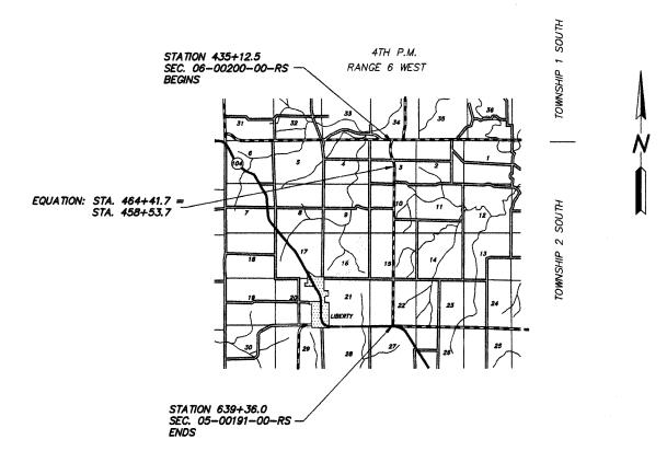
PROPOSED IMPROVEMENT CONSISTS OF PLACING 2" POLYMERIZED HOT-MIX ASPHALT SURFACE COURSE, MIX "C", N50 ON THE EXISTING 22' ROADWAY WITH OTHER MISCELLANEOUS CONSTRUCTION
