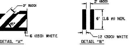
TYPICAL CROSSWALK MARKING
