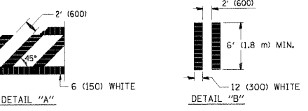
TYPICAL CROSSWALK MARKING
