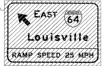
COVER SIGN PANEL FOR EXIT TO RAMP 55S64E
