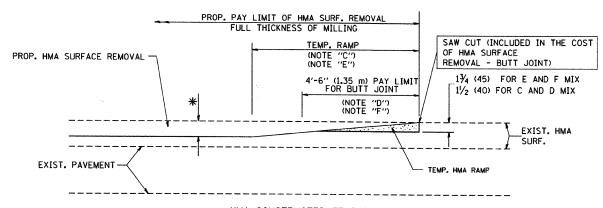
HMA CONSTRUCTED TEMPORARY RAMP
