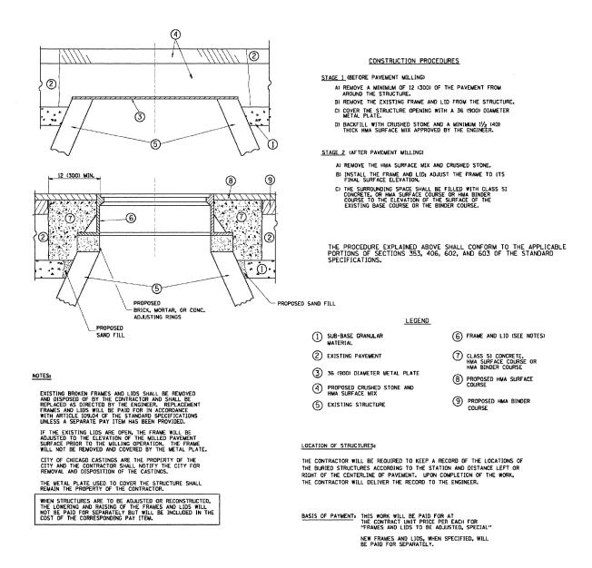
DETAILS FOR FRAMES AND LIDS ADJUSTMENT WITH MILLING
