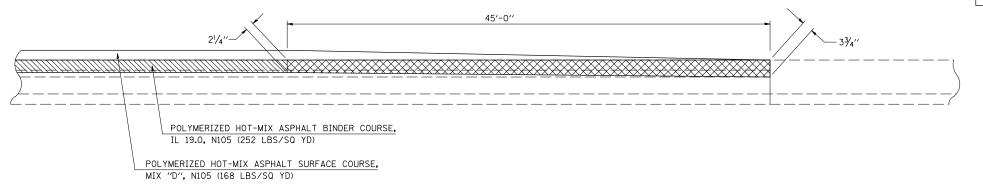
HOT-MIX ASPHALT SURFACE REMOVAL - 21/4"
