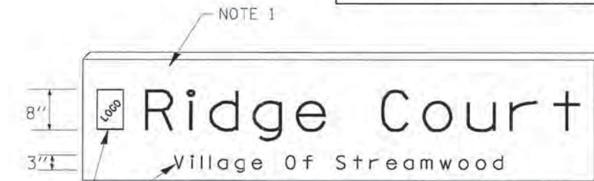
LED ILLUMINATED SIGN PANEL 8'0 x 2'6" (750 mm x 2.5 mm)(MAX) C or D FONT
