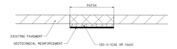
THE CA 6 OR CA 10 SHALL BE COMPACTED IN A MANNER APPROVED BY THE ENGINEER. IF THE MOISTURE CONTENT OF THE MATERIAL IS SUCH THAT COMPACTION SATISFACTORY TO THE ENGINEER CANNOT BE OBTAINED, SUFFICIENT WATER SHALL BE ADDED SO THAT SATISFACTORY COMPACTION
