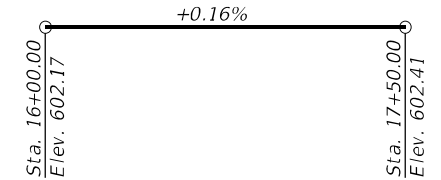
PROFILE GRADE (along centerline roadway)
