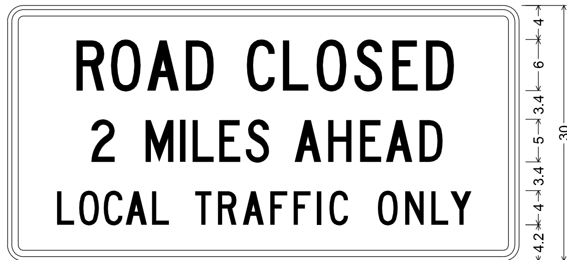
M6-1(R); 1.5" Radius, 0.6" Border, 0.4" Indent, Black on Orange; Standard Arrow Custom 14.6" X 7.0" 0°;
