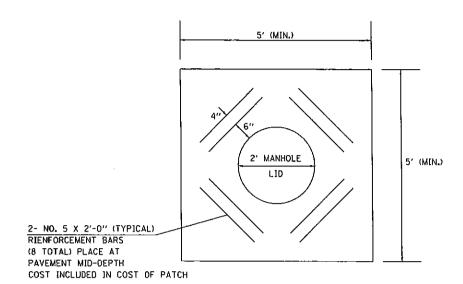
PATCHES SHALL BE 10" IN DEPTH AND CONSTRUCTED ACCORDING TO HIGHWAY STANDARD 442201-03 AND SECTION 442 OF THE STANDARD SPECIFICATIONS
