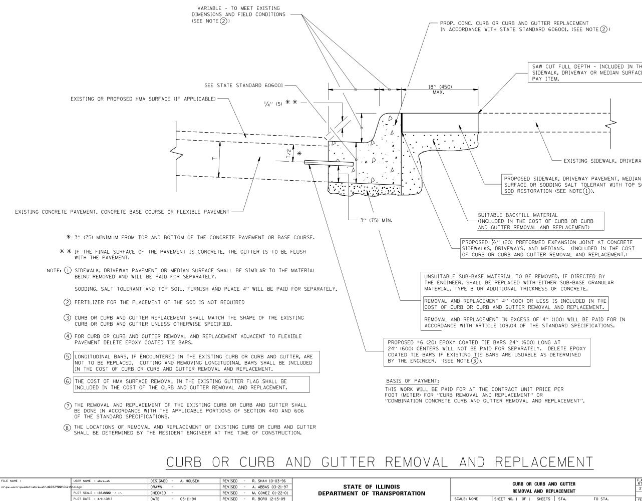
SAW CUT FULL DEPTH - INCLUDED IN THE COST OF SIDEWALK, DRIVEWAY OR MEDIAN SURFACE REMOVAL
