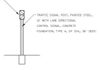
DETAILS OF SECONDARY SIGNAL STA. 31+33.87
