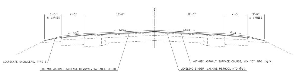
HOT-MIX ASPHALT SURFACE REMOVAL, VARIABLE DEPTH
