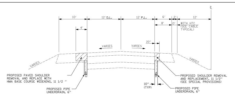
NOTE: TO PROVIDE ADEQUATE DRAINAGE FOR THE PIPE UNDERDRAINS INTO THE MEDIAN DITCH, PLACE THE FLOWLINES OF THE PASSING-LANE-SHOULDER PIPE UNDERDRAINS AT THE DEPTHS SHOWN FOR THE FOLLOWING LOCATIONS. AT ALL OTHER LOCATIONS, THE DEPTHS SHOULD BE 24". DEPTHS ARE MEASURED FROM EXISTING PAVEMENT.
