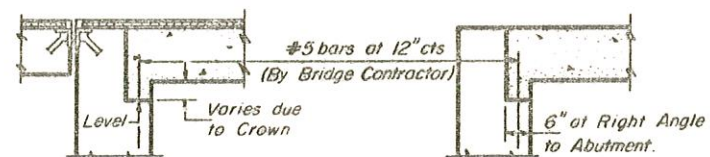
(When bituminous surface is being placed on bridge and approach.)
